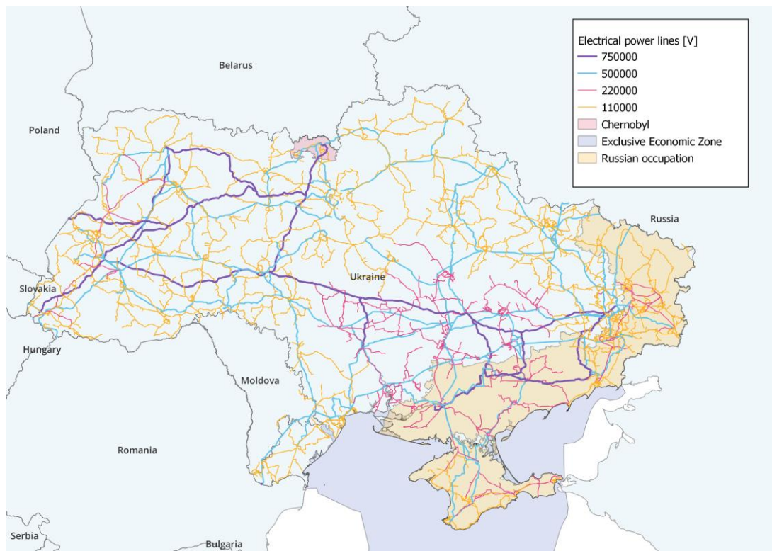
Figure 8: Ukraine's electrical power network (Source: own illustration compiled using PyPSA-Earth (Parzen et al. 2022))
